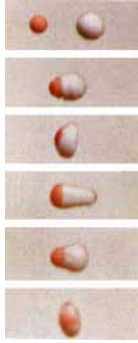
FIGURE 23. Head-on coalescence collision of two unequal-size drops at \Delta = 0.6 , and We = 25 .
