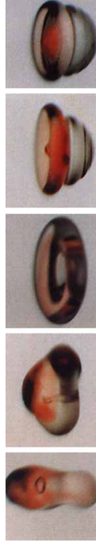
FIGURE 24. Air entrapment during the coalescence collision of two unequal-size drops at \Delta = 0.65 , We = 30 , and x = 0.05 .
